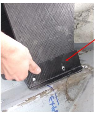
Position the 90' carbon lower bracket along the bottom inside edge on elise S2 (outside i.e behind on Exige S2) and Then mark the hole positions required in the mount to match those in the floor of the boot (Elise and Exige are different, See section G). Next drill 8mm holes in the base. Then bolt the bracket in place to the supports and boot floor/chassis. (ELISE CLAM SHOW!)
