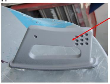
Now drill through the 4 clamshell mounting holes into the carbon curved 90' support of the internal carbon/foam boot strengtheners. Inject some silicone into the top 4 clamshell holes to stop water ingress. Stick some 3mm self adhesive neoprene to the underside of the alloy supports and trim around with a sharp knife. Next bolt the alloy supports in place and refit the wing.
