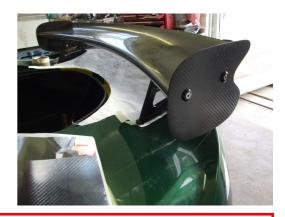
WITH THE VEHICLE ON A FLAT SURFACE AND THE RIDE HEIGHT EQUAL ALL-ROUND, SET THE WING TO THE ANGLE OF ATTACK YOU REQUIRE. TUNE THIS AT A RACE CIRCUIT OR WIND TUNNEL TO GIVE A NEUTRAL AERO BALANCE. NOTE ADD APPROX 2 DEGREES TO THE READING AS IT SHOULD BE TAKEN TO THE CENTRE OF FRONT WING RADIUS NOT TOP.
