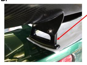
Bolt the Alloy Wing mounts to the wing at a mid angle of attack position. The wing supports outer sides should be approx 909mm apart. Then sit the wing and supports carefully on the boot, Centralise the wing on the boot using the lines on the template as reference to help. Check the boot can open if using the curved wing profile. Check the holes marked are in the right position if not then re-mark them in a new position you are happy with.
